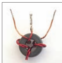
Fig. 3: Windings transformer T2 on a T37-61 core with 2+2 turns (25s.w.g.) bifilliar wound. the end of one winding is connected to the start point of the other.
