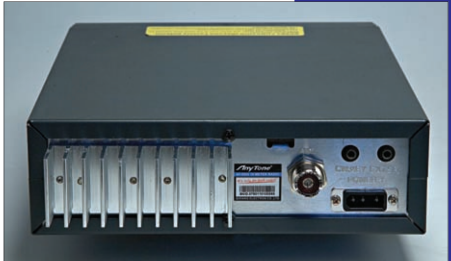
Fig. 2: The rather spartan back panel, has little more than a d.c. power socket, an SO-239 antenna socket and two 3.5mm jack sockets, one for the external speaker and the other for a Morse key.
