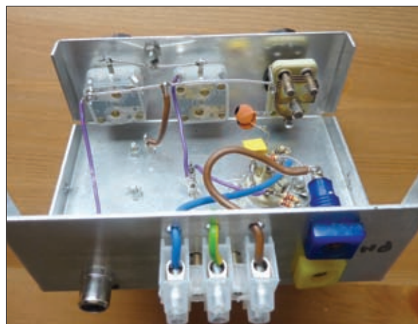
Looking at the underside of the one-valved receiver chassis, you could make the chassis up out of soldered-together p.c.b. material, if you have some to-hand.
