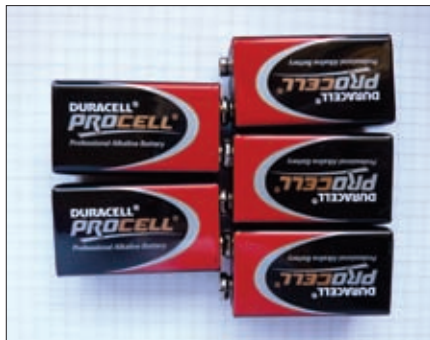
Fig. 5: Combining five 9V batteries together to make a 45V supply
