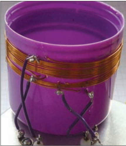
Fig. 3: After looking around the house for a suitable coil former, George found one with the right diameter of about (50mm) in a soft plastic material – a furniture polish spray-can lid! L1 is 10 turns, and L2 is five turns, with a 3mm gap between them.
