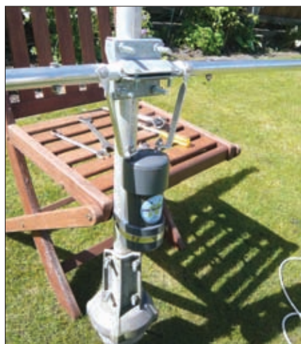
A close up view of the central insulating rod, matching transformer and rotator in their final positions.
