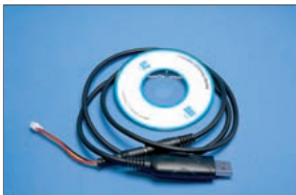
Fig. 4: The programming interface and software CDROM. Unusually you have to remove the covers, to fit the interface into a small p.c.b. mounted socket just visible to the right of the upper flat ribbon cable in Fig. 3.
